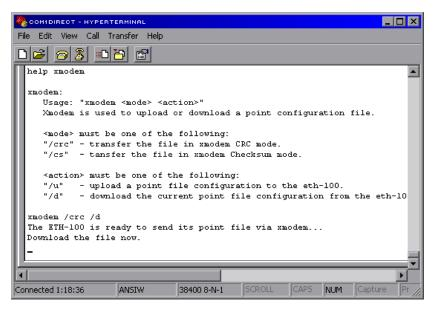
Figure 16: "xmodem" Command Overview and Implementation
